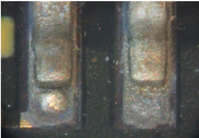
Poor solderability and de-wetting on toe joints
