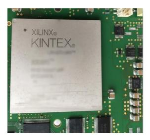
Retronix's advanced, precise and safe component recovery service was used to recover the high value part from the faulty boards. There was no room for error because of the overall value of the component and the critical application. Retronix successfully recovered, laser reballed, tested (electrically and mechanically), vacuum packed and sealed the parts and shipped them to the customer. With positive feedback —
